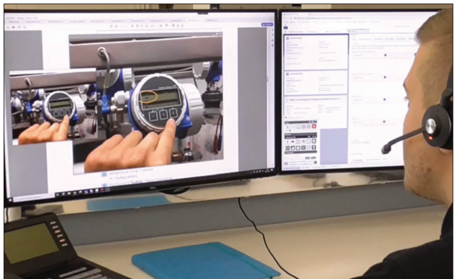
Figure 1. Using an augmented reality application, support engineers can see everything the technician sees in the field, and then guide troubleshooting or maintenance efforts using a virtual pencil to highlight target components for the technician.
