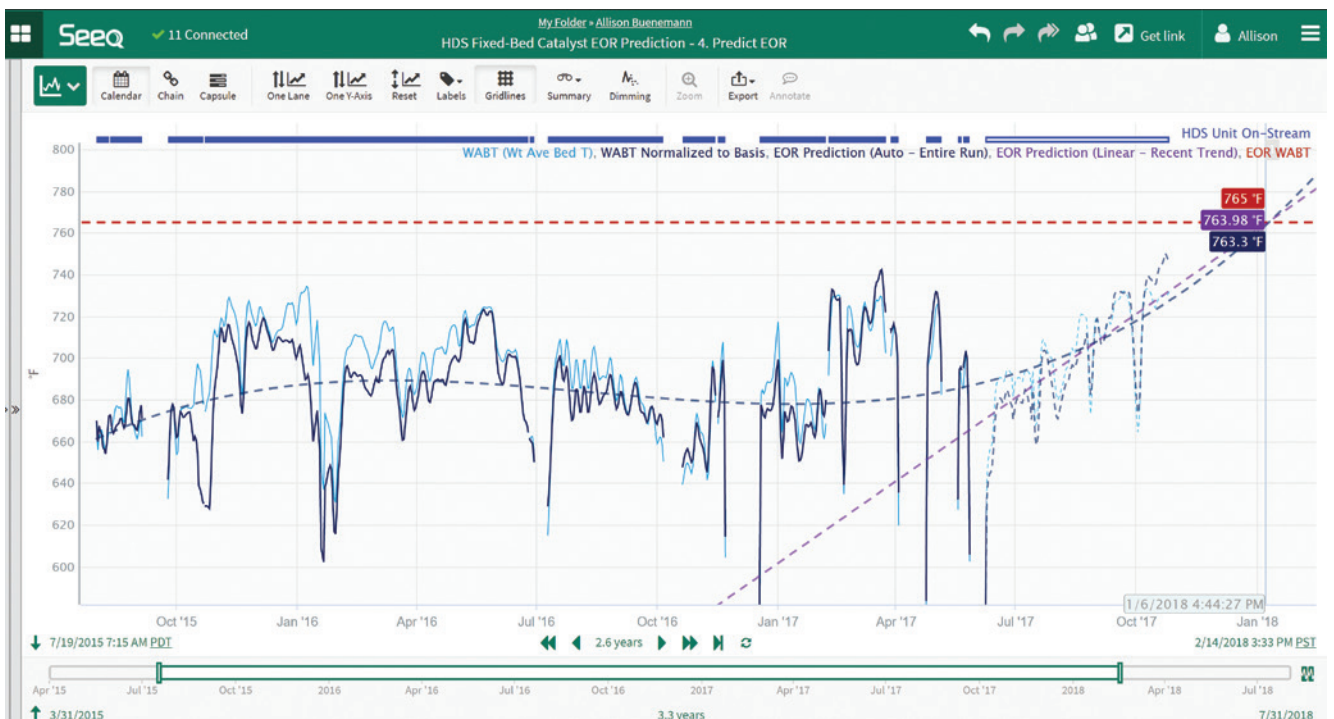
Figure 3. Using the advanced analytics application, SMEs compared WABT predictions from a full data set to a recent sample to determine maintenance requirements in the coming months.
