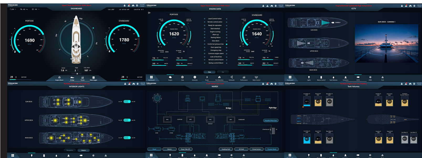
Figure 3. These HMI/SCADA dashboards and displays are developed as templates to provide a quick start for marine designers.
