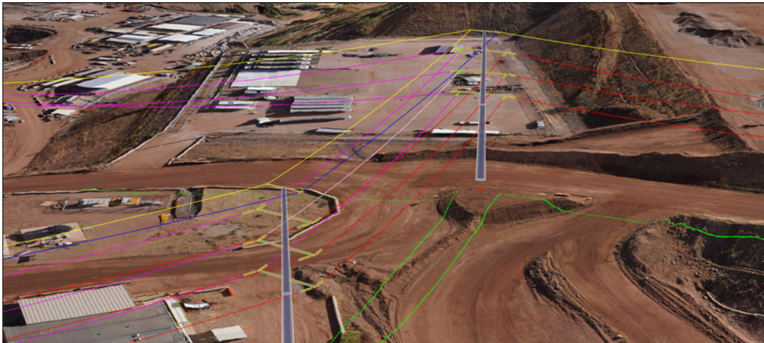
After applying AI to create a model of an area, other layers can be added, such as future electric wiring (pictured here) or a conceptual hauling/charging infrastructure option.
